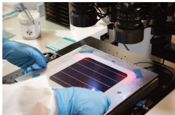
Oxford PV puts a thin layer of its perovskite material on the top of standard silicon solar cells to convert significantly more of the sun’s energy into electricity. Image credit: Oxford PV.
