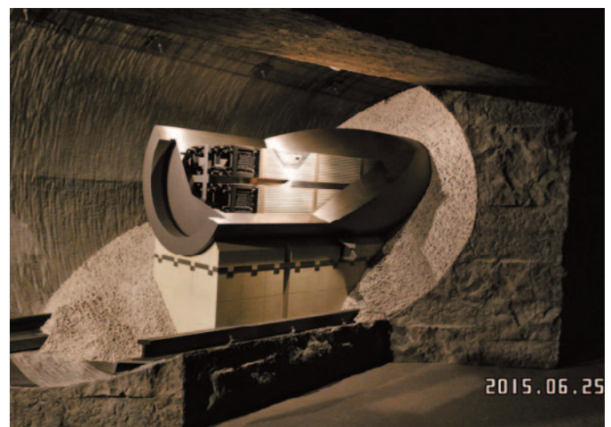
Figure 3: Illustration of spent fuel disposal system, using a carbon steel container surrounded by a clay buffer, in a lower strength sedimentary rock, at the Mont Terri underground laboratory in Switzerland.
