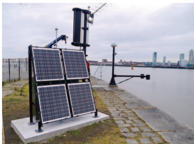
The new NOC tide gauge at Liverpool, Alfred Lock (courtesy of Geoff Hargreaves, NOC)
