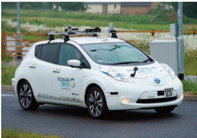
The Government-backed HumanDrive project, led by Nissan, developed an advanced, automated vehicle system that emulates the natural driving style of a human at the wheel. The project culminated in a successful 230-mile fully self-driving demonstration from Cranfield to Sunderland in 2019.
