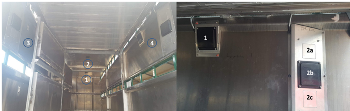
Fig. 1. (A; LEFT) ceiling mounted (1) and (2) in front compartments and wall antennae (3) and (4). (B; RIGHT) wall antennae (1) fixed and (2) adjustable into 3 positions (a, b or c).
