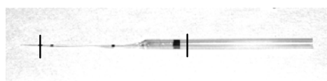
Figure 1 (above) CryoTips used in the present study were sealed at positions indicated by the vertical lines.
